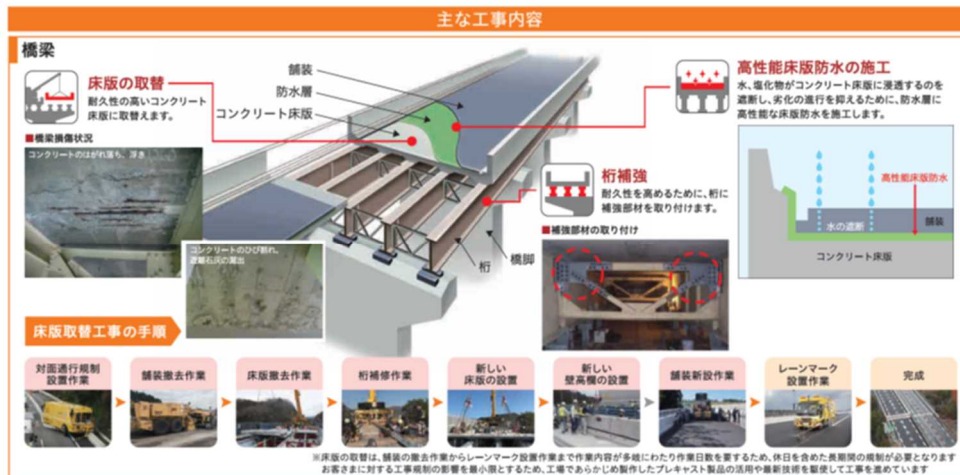
Figure 3: Detailed Construction on Bridge Slabs 6
