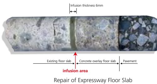
Repair of Expressway Floor Slab
